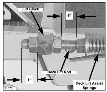
Left Rod Protruding Threads Figure 3-20
